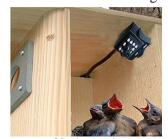
It's a color camera with built-in Infrared (IR) lighting that switches on automatically in the dark. It's 1.75" x 1.75" x 1" and fits nicely in the corner of the two owl boxes I have. I bought the first one in May, 2019 and discovered that it puts out standard Audio/Video via RCA jacks so I had to also order a *Hauppauge 610 USB-Live 2 Analog Video Digitizer* that would allow me to record movies or snapshots onto my laptop.
